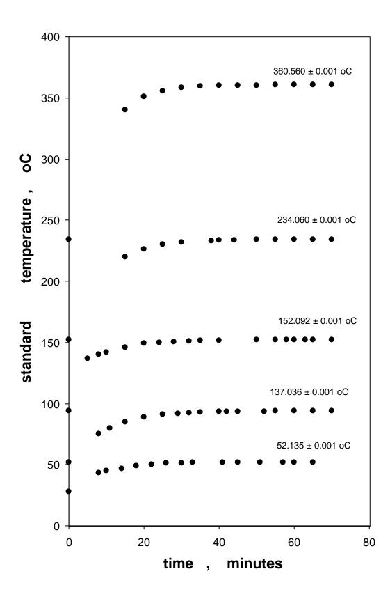
Kinetic curves obtained on the experimental model of ISOCALT 21/70/3 for successive temperature steps.
