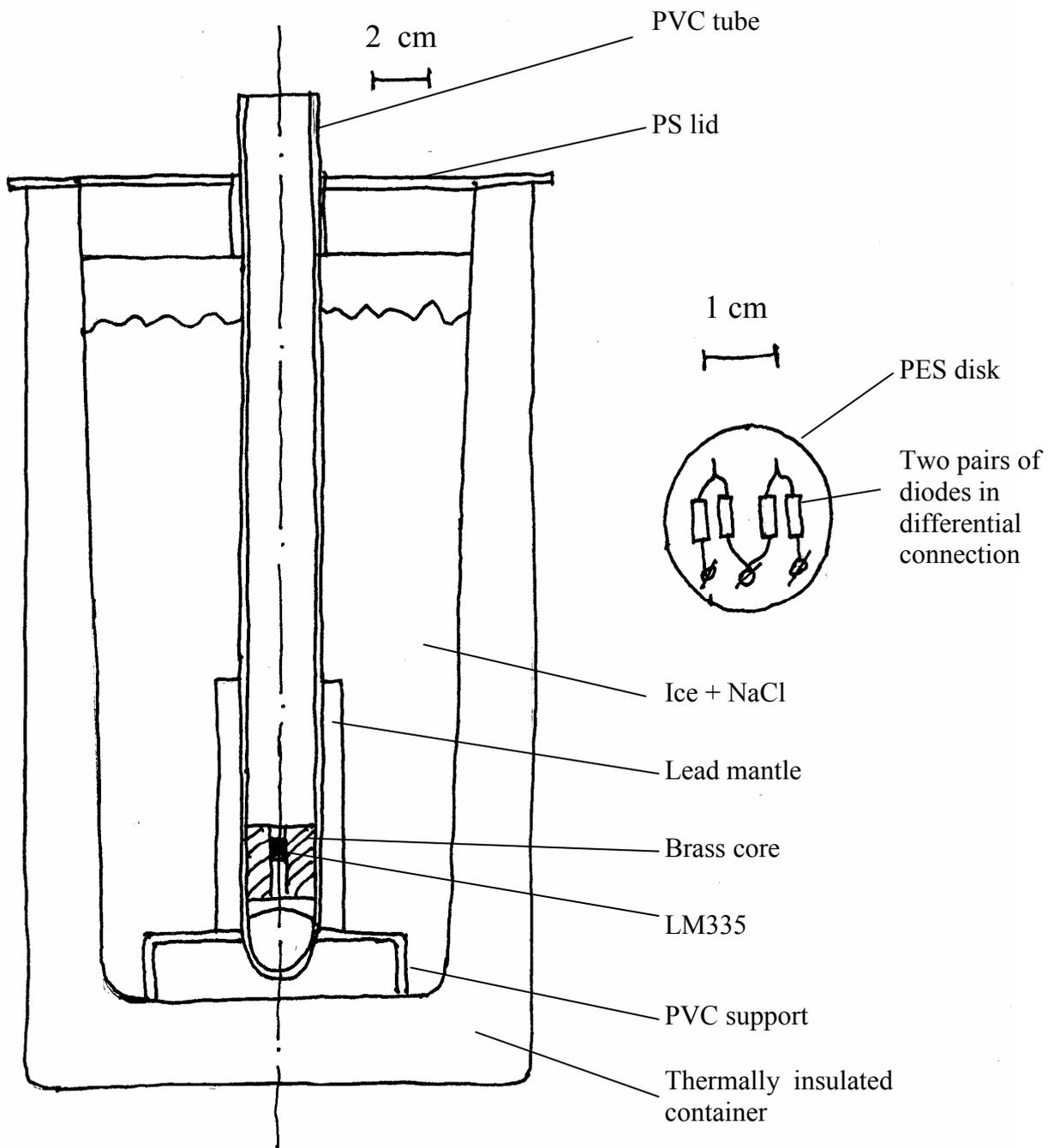
Figure 1. Cross section of DTA disposition with details for T and dT sensors.
